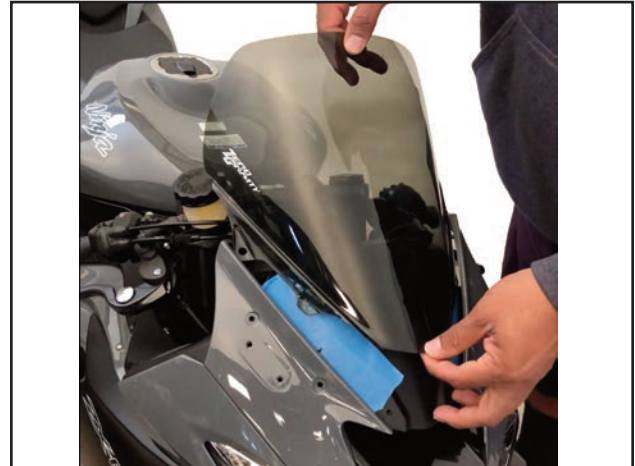
Part 4 Pulling the upper fairing inserting ZG screen
