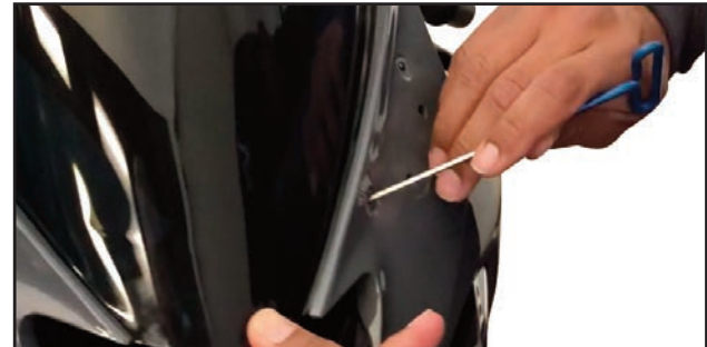
Part 5 Wellnut alignment & inserting allen screws to finish install
