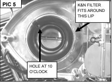
STEP 11 Refer to PIC 5. Align the black plastic Dual Velocity ring with the Hypercharger vent hole. Press it all the way into place. The ring will "snap" into place.
