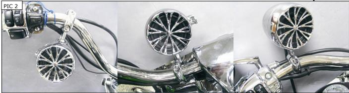
STEP 4 Remove the screws from the clamp, install the clamp on the handlebars, and make sure that no wires are being pinched; place a small amount of anti-seize to the screws and reinstall them, only tightening them enough to prevent the clamps from rotating. PIC 3
