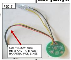
STEP 3 Connect the short yellow and black wires from the Deco Fuel Gauge to their corresponding wires
