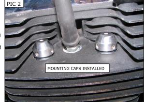
STEP 5 Holding the Cover centered in the spark plug opening and sitting level to the head, tighten the cap screws securely. PIC 4
