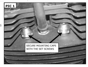
Refer to PIC 2. Determine the Front and Rear Bahn Spark Plug Head Bolt Covers.
