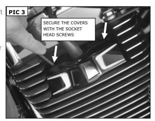
STEP 5 Holding the cover centered in the spark plug opening and sitting level to the head, tighten the Socket Head Cap Screws securely.
