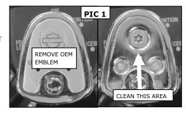
STEP 4 Test fit the BAHN Ignition Switch Cover over the ignition switch. Note the alignment of the
