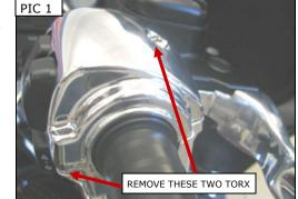
**STEP 3** With the switch housings separated, slide the stock handgrip assembly off the handlebars. This will not be re-used.
