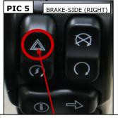
HAZARD (4 WAYS) BUTTON ON HAND CONTROLS = CAN BUS SYSTEM
