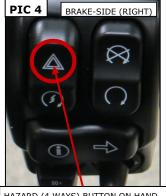
HAZARD (4 WAYS) BUTTON ON HAND CONTROLS = CAN BUS SYSTEM
