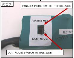
USE INCLUDED LOAD EQUALIZER FOR PANACEA, LED CONVERSIONS OR NO OUTBOARD REAR TURN SIGNALS
