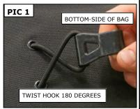
Refer to **PIC 1**. Secure the bag to the existing luggage rack with the two bungee hooks. Twist the hooks 180 degrees so the hooks face upward.
