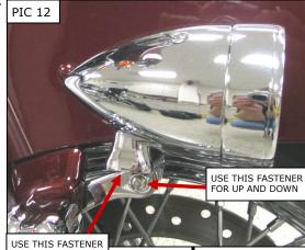
ENSURE THAT THE INSTALLATION OF THIS PRODUCT DOES NOT CONTACT ANY OTHER COMPONENTS, ESPECIALLY MOVING/ROTATING COMPONENTS (WHEEL, TIRE, VALVE STEM, WHEEL WEIGHTS, ETC.). CONTACT BETWEEN MOVING AND STATIONARY COMPONENTS CAN CAUSE DAMAGE LEADING TO LOSS OF CONTROL RESULTING IN SERIOUS INJURY OR DEATH.
