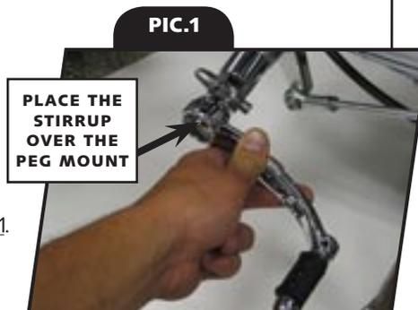
**STEP 4** Place the splined end of the existing Liberator peg into the new Stirrup. See [PIC.2](#).
