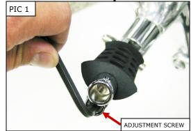
**WARNING** FOOTPEGS MUST BE INSTALLED SO THEY WILL FOLD UPWARD AND REARWARD IF HIT BY ANY OBJECT. FAILURE TO ADJUST THE FOOTPEGS TO OPERATE IN THIS MANNER COULD RESULT IN SERIOUS INJURY OR DEATH.
