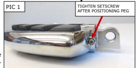
STEP 3 Install the new peg using any spacers or washers removed in Step 2. Line up the hole on the male mount on the new peg with the hole in the clevis.
