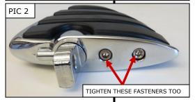
FOOTPEGS MUST BE INSTALLED SO THEY WILL FOLD WARNING UPWARD AND REARWARD IF HIT BY ANY OBJECT. FAILURE TO ADJUST THE FOOTPEGS TO OPERATE IN THIS MANNER COULD RESULT IN SERIOUS INJURY OR DEATH.
