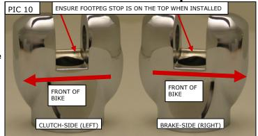
NOTE: Place a drop of Loctite Threadlocker Blue 248 on the threads of the clevis and footpeg screws before installing. Follow the manufacturer's recommendations for proper application.
