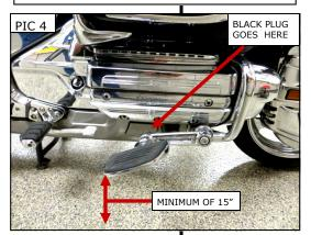
• Rotate the clevis and Mini Board assembly to the desired angle then push the assembly back into the swingarm, making sure the roll pins in the clevis line up with the holes on the swingarm, and re-tighten the fasteners. Install the black plastic thread plug in the swingarm. PIC 4
