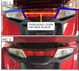
ATTENTION! The adhesive will not bond correctly if applied at temperatures less than 50°F. Do not attempt this installation in temperatures less than 50°F.
