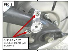
**ATTENTION!** Determine a mounting location and orientation of the mount before fully tightening the fasteners. The mount may leave marks when tightened down.
