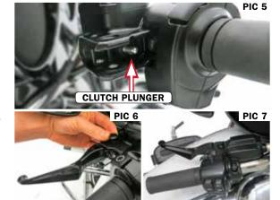
STEP 7 Refer to PIC 6 and 7. Reinstall the pivot pin and secure with the snapring. Tighten the clutch (left) side handlebar switch housing assembly screws. Compress the Clutch Lever a few times to ensure that the clutch works properly BEFORE starting the motorcycle.
