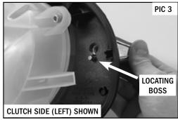
STEP 9 Place the Left Rubber Spacer (with the angled side facing inward) over the Mount locating-boss; align the holes. Refer to PIC 4
