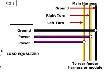
Load equalizers generate heat when in use. Avoid using the turn signals CAUTION for an extended period of time, otherwise the load equalizer will overheat. Never operate the four-way flashers unless you first remove the load equalizer. Overheating will damage the load equalizer, causing loss of turn signal operation and may create a fire hazard!
