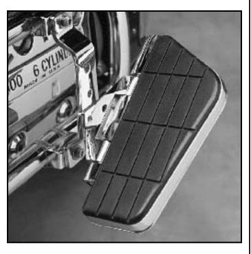
4. Install anti-swivel bracket (Item #3) and floorboard (Item #4) onto bar, using <sup>5</sup>/16" bolt and star washer (Items # 9, 10). Install through one of three holes that provides desired ride height.
