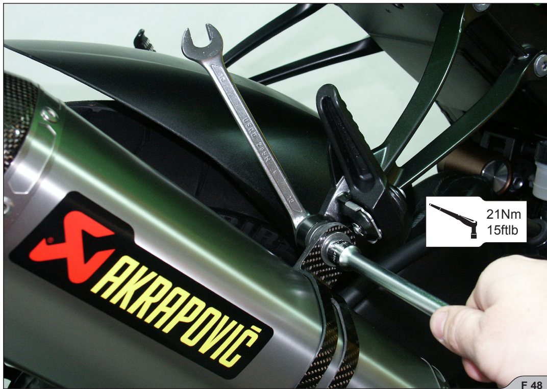
13. Tighten the metal clamp of link pipe/collector joint (F 49).
